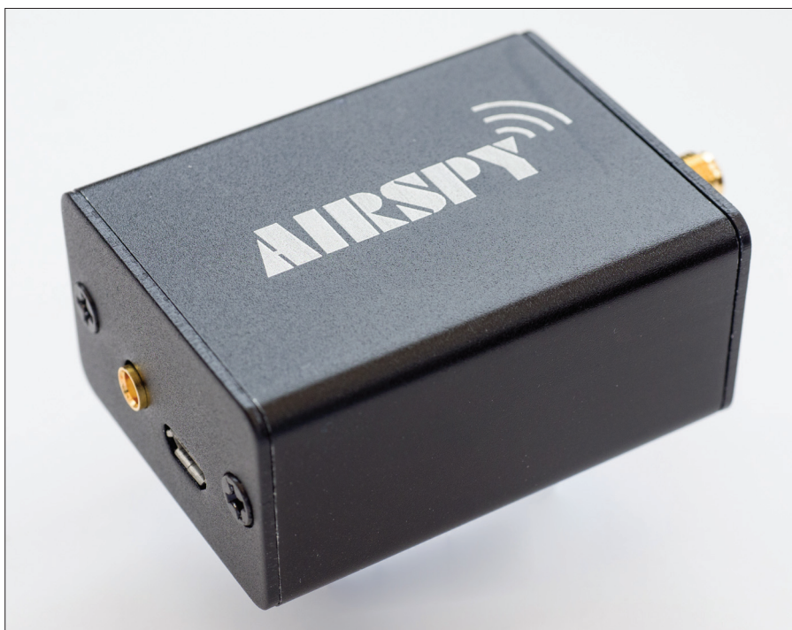
The Airspy wideband SDR receiver.
