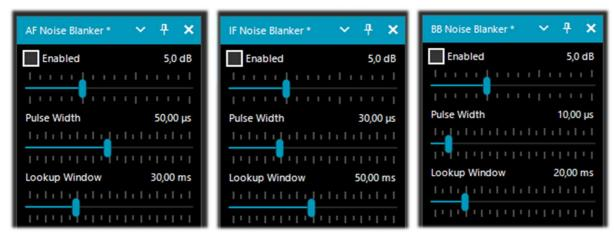
There are obviously no preset values or thresholds, so you need to gradually move the various sliders until the pulsing noise disappears or reduces without distorting too much the received audio.
