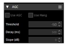
In WFM mode the AGC is disabled because the FM signal is limited and its amplitude is constant. For NFM the AGC acts on the Audio output. This is useful with weak signals with low modulation index. For AM, SSB, CW and RAW, the AGC acts on the narrow band IF, as usual.
