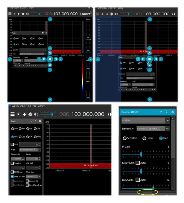
Since release 178x, the panels have an automatic scrolling function on the right, or for resizing, the little horizontal bar (highlighted in yellow) can be used with the mouse. At this point, if you like the composition, you can decide to save the layout with a name of your choice so that it can be loaded later using the items in the hamburger menu: "Save Layout... and Load Layout...".
