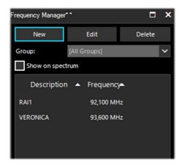
Then a double click on a record will tune SDR# to that frequency, automatically setting the emission mode and its bandwidth. If the "Show on spectrum" box is checked, the frequency label will be displayed in the RF spectrum.
