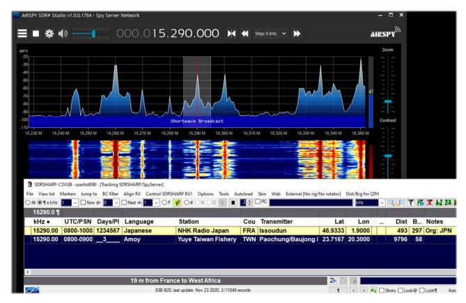
In this screenshot, a Spy Server Network is used to verify a broadcaster on 19-meter. By enabling the "Track mode" option, the first line appears in CSVUB with its transmission highlighted. For very busy slots, you could also use the "Now" option which immediately filters the transmission at the current time. Let's see in detail the possible plugin configurations through the "databridge".
