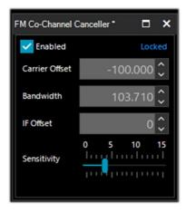
Example: strong WFM station at 91.500 MHz and weak station tuned to 91.600 MHz (red vertical center BW line at about 100k).
