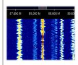
This window shows the graphic representation in real time of the intensity of the received signals as a function of frequency (on the horizontal axis) and time (vertical axis) with the new data represented in cascade starting from the top and going down: hence the name waterfall.
