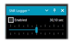
Once the flag has been enabled and a time interval has been selected with the cursor (up to 60 seconds), a text file with a name similar to this one will be created in the program directory: "SDRSharp\_20210205\_153455Z\_SNR.csv" in which the SNR values (in dB) detected by the active frequency in the VFO will be recorded. The file can be imported into Excel for further analysis.
