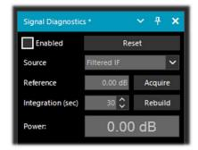
On YouTube, the radioamateur Leif Asbrink (SM5BSZ) has uploaded some very interesting and technical videos, where he shows how the AIRSpy HF+ can be used as an accurate power meter for RF signals. He points out that if the noise figure (NF) or minimum distinguishable signal (MDS) of a device is known, then it is possible to use this device as a power meter by calibrating it with a resistor (dummy load) at room temperature.
